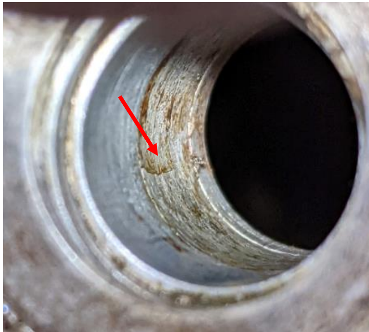
Figure 9. Example of Corrosion in Bolt Hole, with Crack PA-28-161, 9,036 hours TIS
